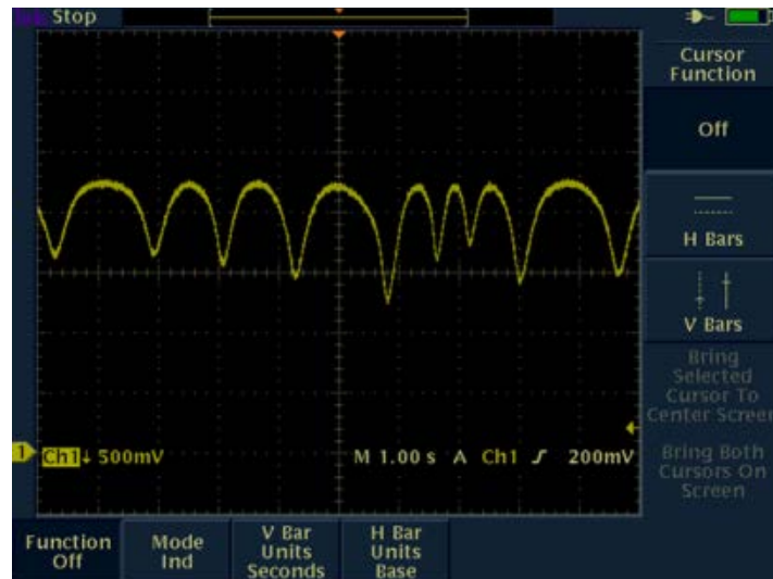
Figure F-10. S-band Telemetry Signal Received from an Aircraft in Flight 65
